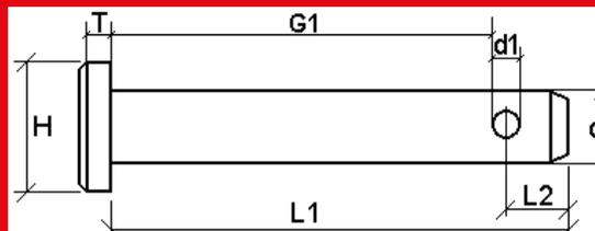
Headed Clevis Pin With A Cross Drilled Hole
